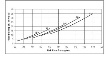
**NOTE:** Total water pressure drop varies depending on a units selected options. Only use the specific chart which reflects your unit. The above figures illustrate total water pressure drop (WPD) for each associated model number.
