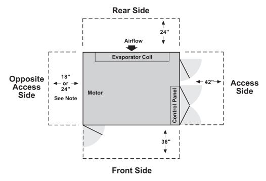
NOTE: If water and condenser drains are on the motor side, 24" is required.
