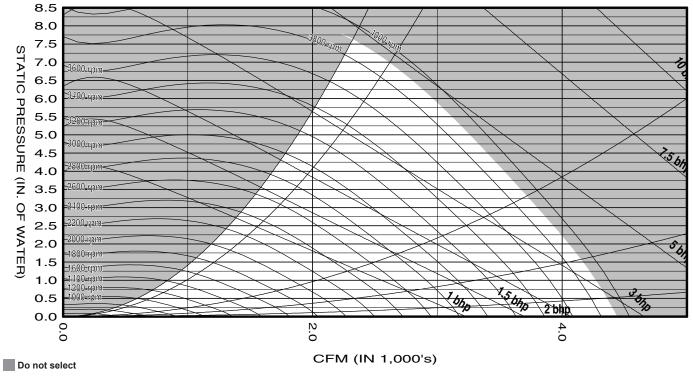
Figure 44: 15.0" Diameter, 9-Blade Fan
